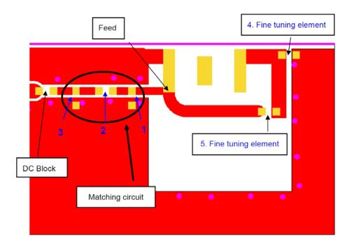
With the following recommended values of matching and tuning components, the center frequency will be about 868 MHz at our standard 80x40 mm evaluation board.
