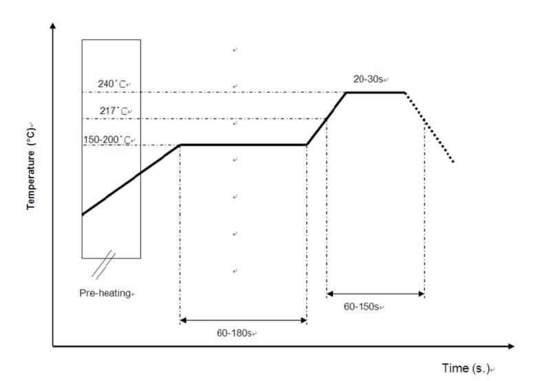
$\label{eq:sacommended} \mbox{\@scale=1.04\eng} Recommended solder paste alloy: SAC305(Sn96.5/Ag3/Cu0.5) Lead free solder paste.$
